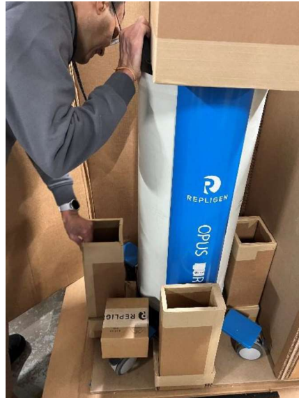
Figure 8. Placement of support blocks
