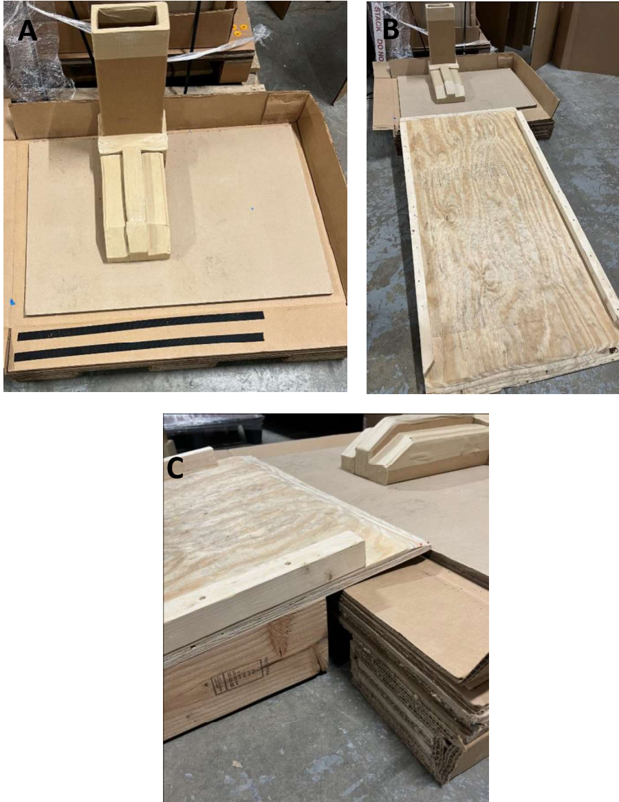
Figure 4. Positioning the ramp
